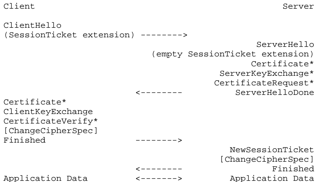
Figure 4: Message flow for server rejecting ticket, performing full handshake and issuing new session ticket
