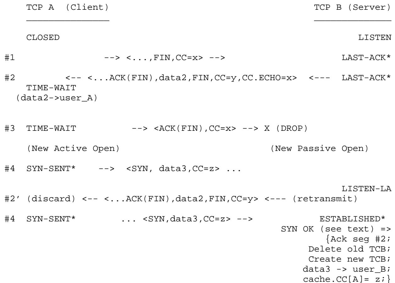
Figure 5: Truncating TIME-WAIT State: SYN as Implicit ACK
