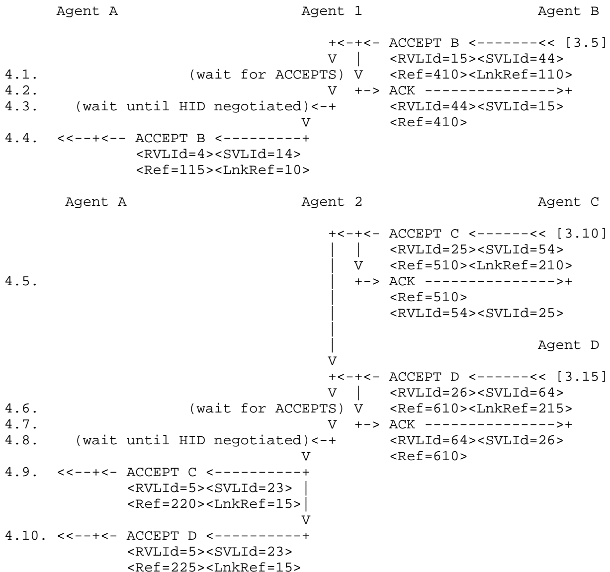
Figure 8. ACCEPT Processing by an Intermediate Agent
